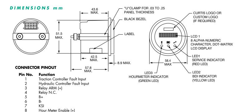
**Note**: In addition to a "U" clamp and thumbnuts/washers shown in the drawing, individually packed units are provided with a mating connector and female pins. Bulk packed units are provided with a "U" clamp and hex nuts/washers only.
