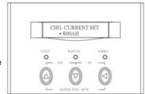
D. Once the correct battery AH is selected, press Enter-key again to save the selection.
