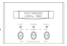
confirm voltage and then the cursor will move to frequency selection. The output frequency (50Hz or 60Hz) can be adjusted by the same key operation.
